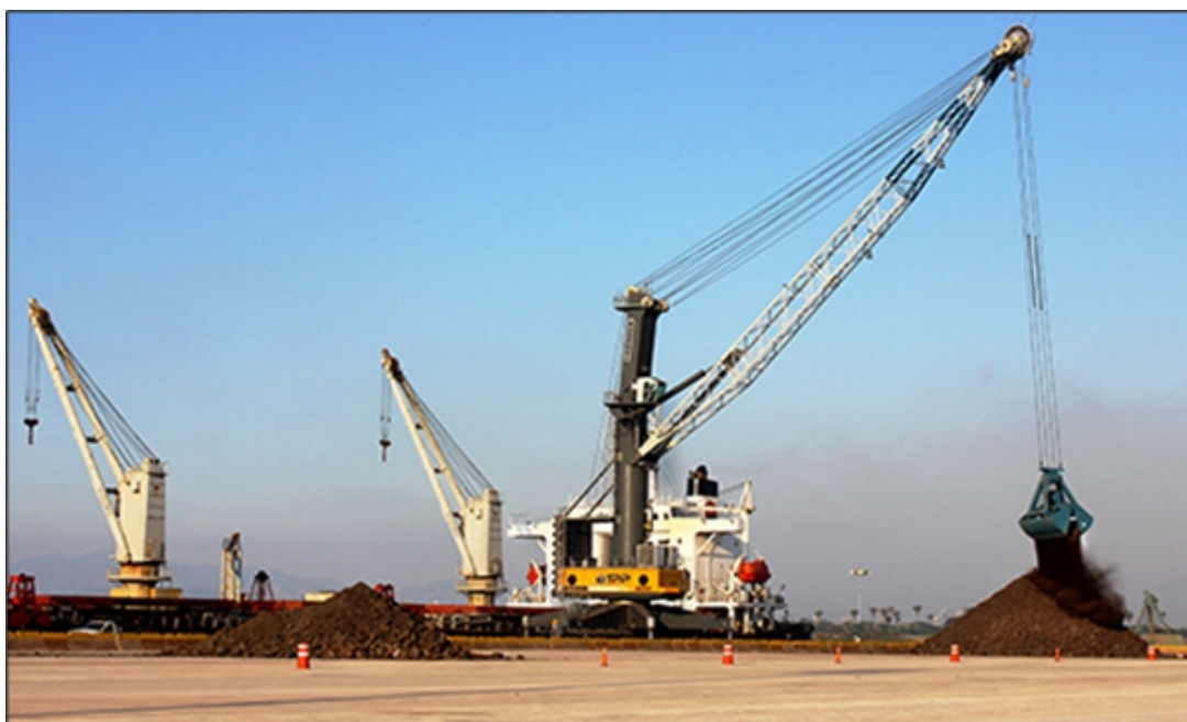
Figure 15.1 Unloading bulk minerals at Mexican port of Lazaro Cardenas (Terminales Portuarias de Pacifico)
