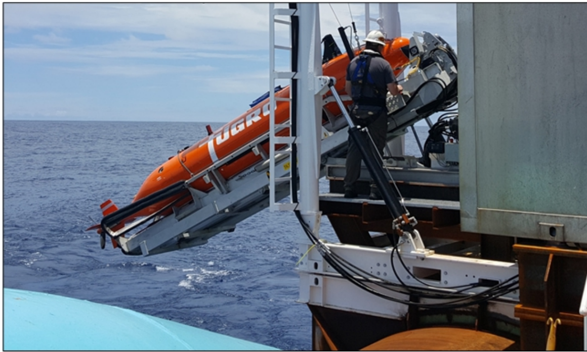
Figure 7.6 Deployment ESVII Kongsberg Hugin AUV from the stern of the Maersk Launcher
