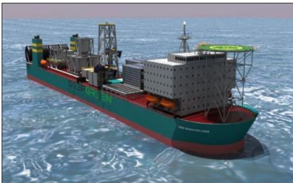
Figure 13.10 Collector Ship 1, production support vessel
