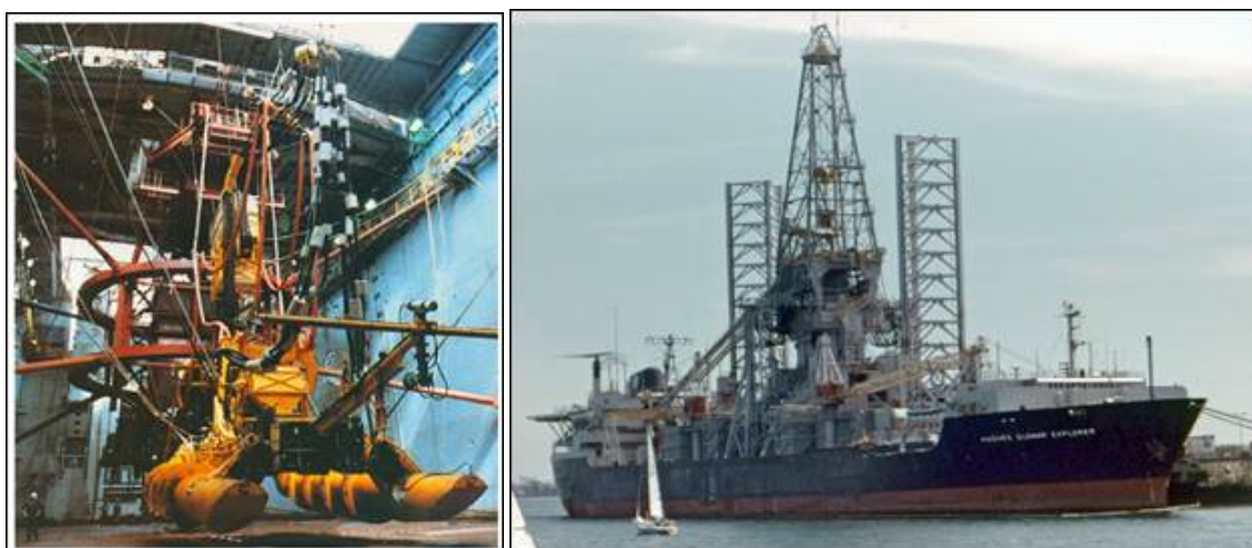
Figure 5.11 OMCO Screw-drive collector and pilot mining vessel, the USNS Hughes Glomar Explorer
