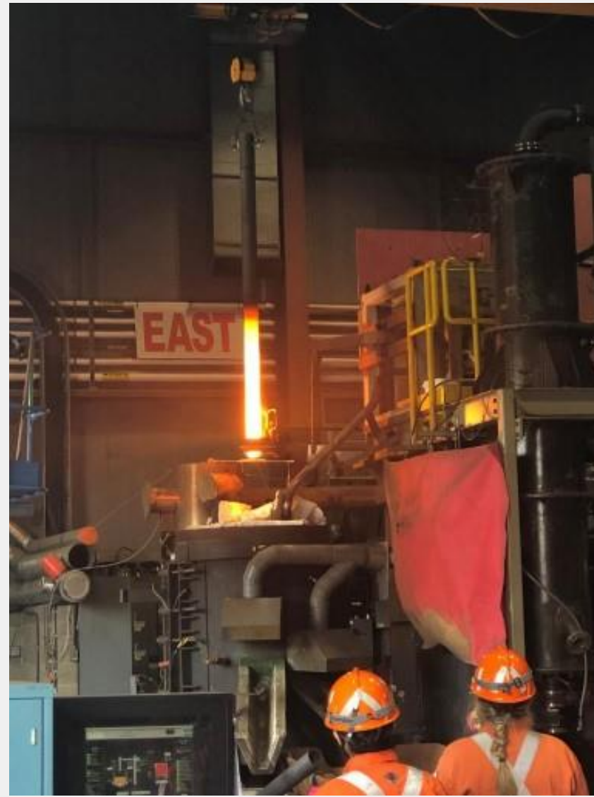
Smelting nodules in an Electric Arc Furnace at XPS facility in Canada. Electrode temperature 1450 degrees C. Smelting results in two products: - Manganese silicate product - NiCuCo alloy (intermediate)
