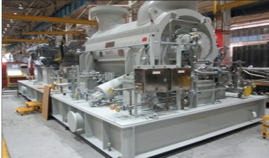
Figure 13.15 Main air compressor (Elliott Group model 46M6I)
