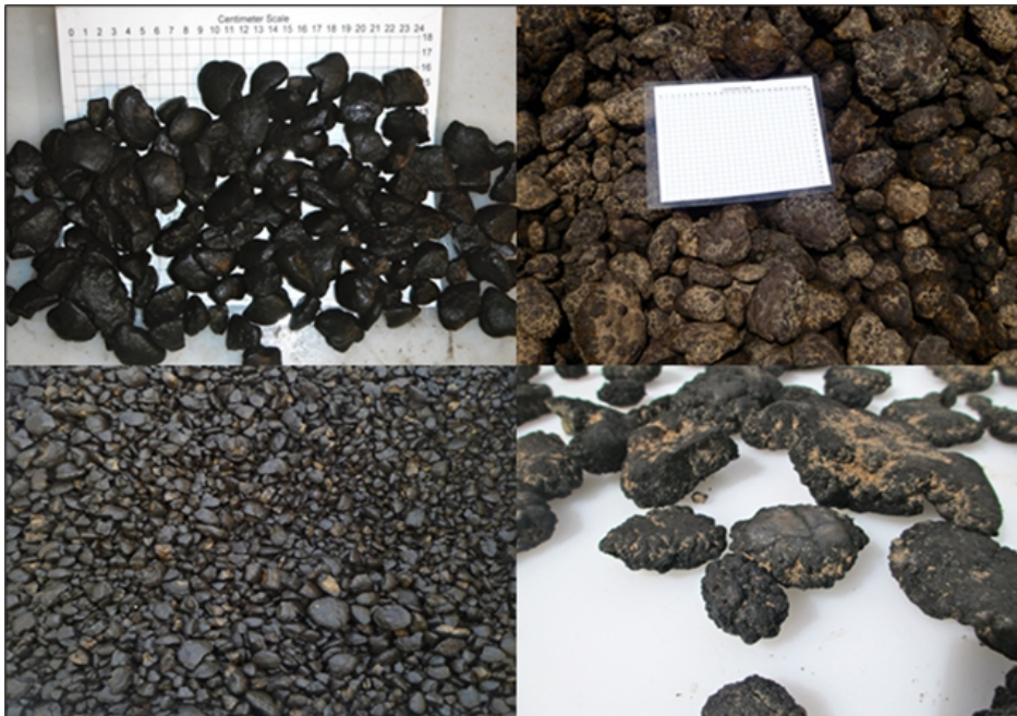
Figure 7.2 Subset of nodule samples recovered during NORI's 2012 exploration campaign
