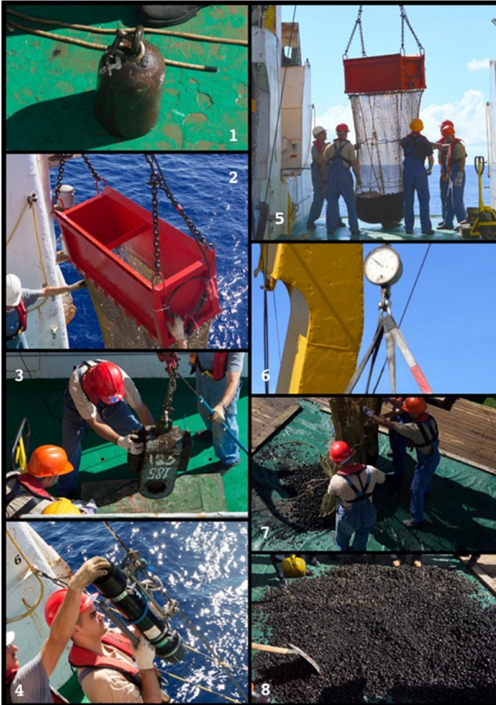
Figure 7.32 Operations and details of the YMG Galatea-trawl dredge
