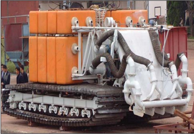
Figure 5.16 Chinese pilot scale tracked and test screw-drive subsea vehicles
