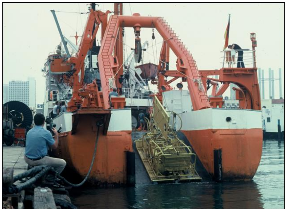
Figure 5.8 INCO electro-hydraulic collector test; DOMCO hydraulic collector launch & recovery test on the RV Valdivia
