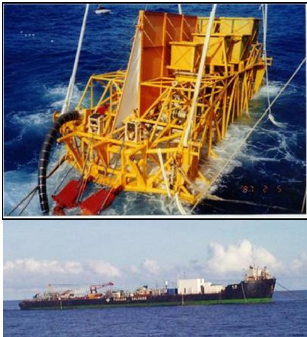
Figure 5.15 1997 Japanese collector, barge and trial schematic
