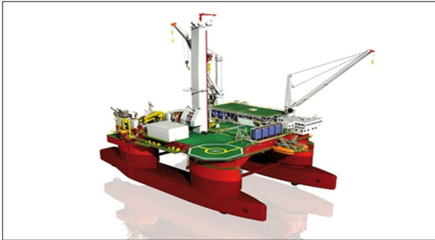
Figure 13.19 Semi-submersible subsea oilwell support vessel, Q4000
