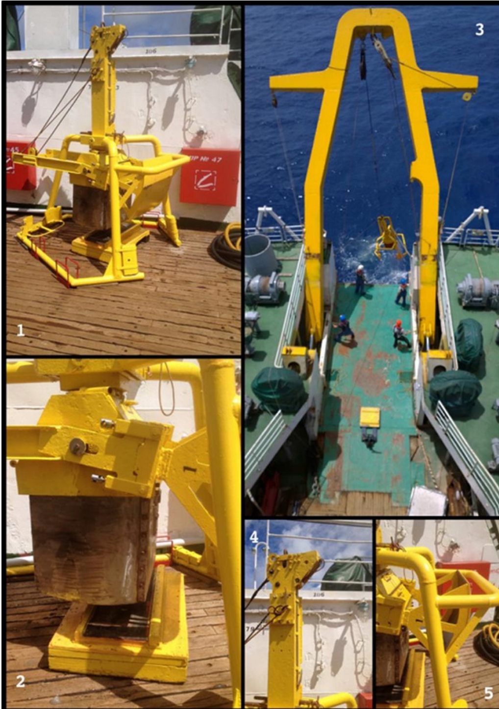
Figure 7.14 Details and recovery of the YMG box-corer
