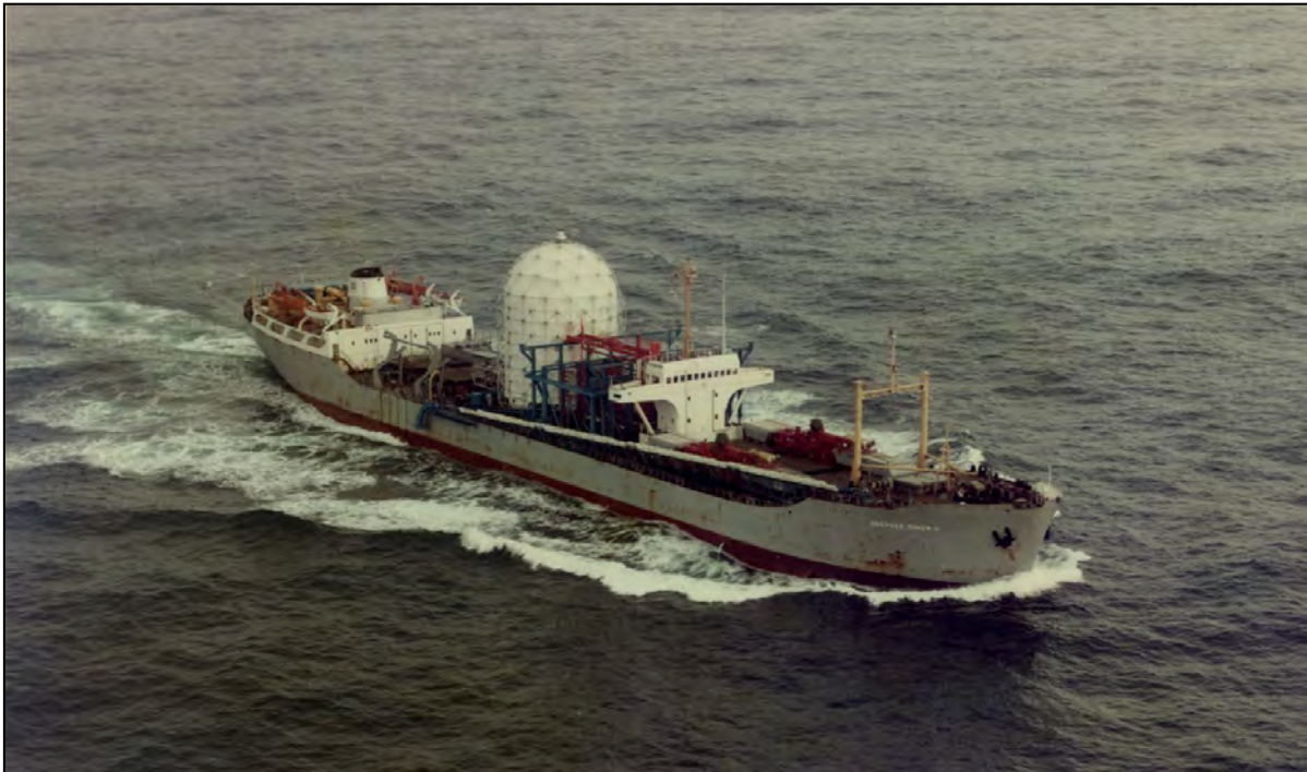
Figure 5.5 Ocean Mining Associate's Deepsea Miner II
