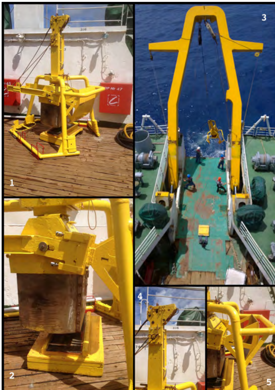
Figure 7.14 Details and recovery of the YMG box-corer
