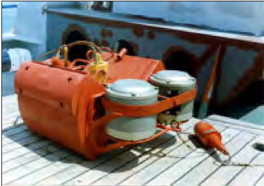
Figure 8.1 Ocean-0.25 Grab Sampler (Yubko, 2012)
