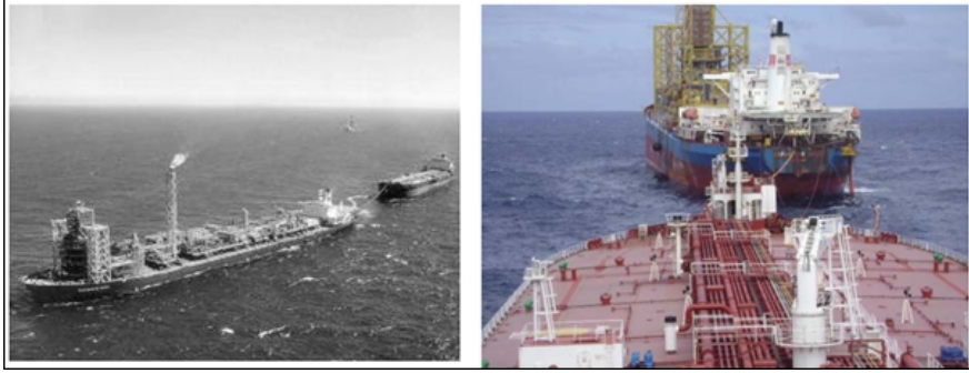
Figure 15.2 Offloading Operation: (left) with a conventional tanker; (right) with a DP tanker
