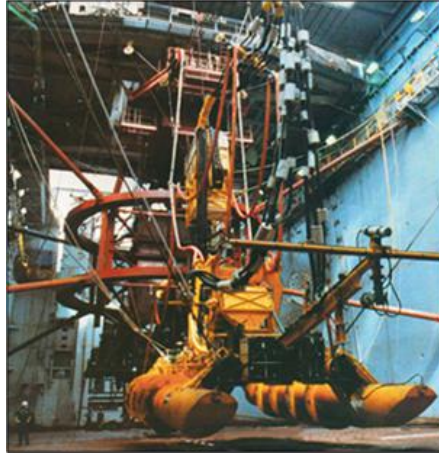
Figure 5.2 Remote operated collector used by the Lockheed Group in 1970s trial mining
