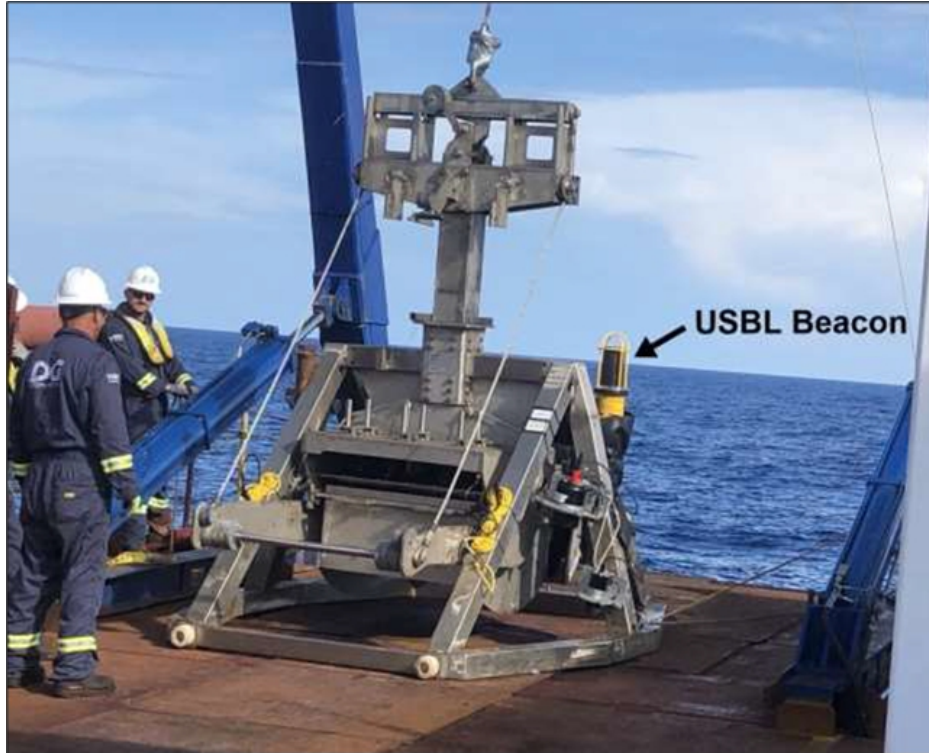
Figure 7.28 Box corer on deck showing the USBL beacon mounting position
