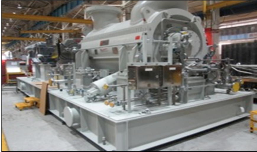
Figure 13.15 Main air compressor (Elliott Group model 46M6I)
