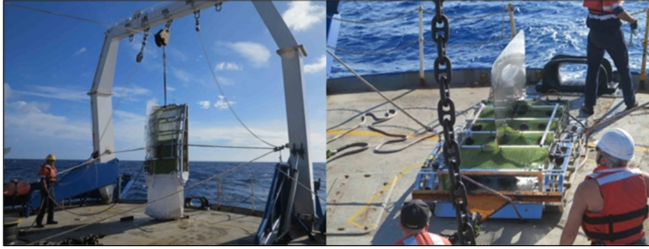
Figure 7.3 Photos showing the operation of the epibenthic sled collecting nodules during the NORI 2013 campaign
