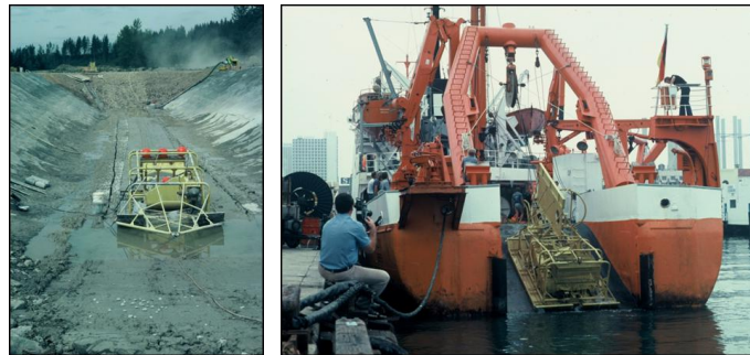
Figure 5.8 INCO electro-hydraulic collector test; DOMCO hydraulic collector launch & recovery test on the RV Valdivia
